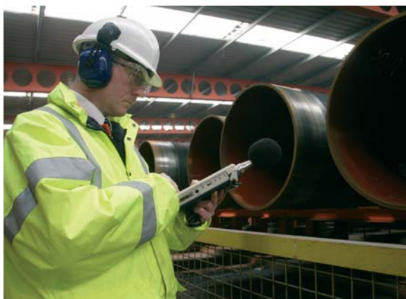
NOISE MONITORING IN AN ENGINEERING WORKS
